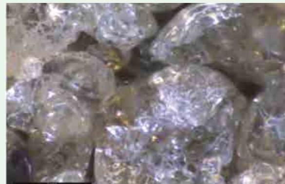
Figure 4: Glassy steel slag produced after metal recovery and slag transformation
