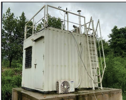
Continuous Ambient Air Quality Monitoring System
